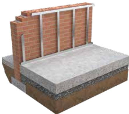
4. Lift the SR019/TB-MF into position using wedges on the floor. Insulation should be cut back to accommodate an adjoining panel at external corners. Joints should be tightly butted.
